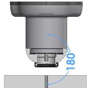
2. The distance between the Screwdriver's bottom part and the surface where the action takes place must be within the range of 0-8 mm.
