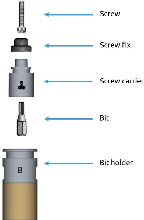
The sections below explain the different components of the Screw-bit System and how to set it up correctly.
